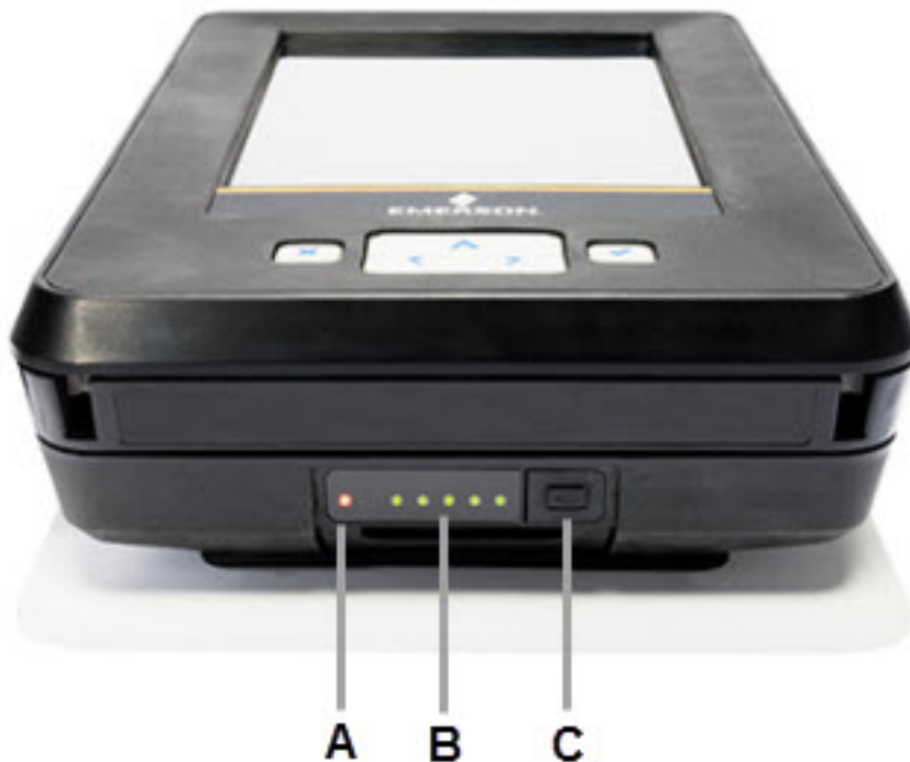
Figure 2-9: LEDs showing approximately 100 percent charge
