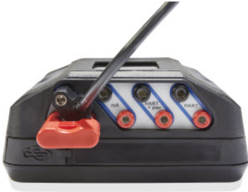
Figure 3-35: FOUNDATION fieldbus Power Plug attached to the Trex unit
